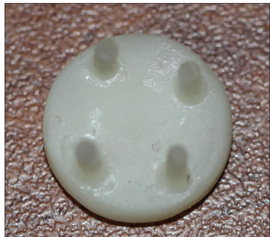
Figure 1: Specimen fabrication with resin cement cylinders on lithium disilicate discs
